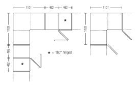
Solution with QUICK and "A FILO" doors (only for corner element 1101x1101)
