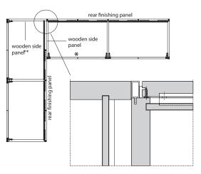
\* This compartment can be closed with a QUICK, "A FILO" and NICHE door (vertical and horizontal). For glass backs, drawer units are mandatory for compartments with frame or glass sides. For melamine structure, piqué or fine grain backs, use drawer units that are narrower than the module.
