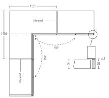
The corner element can be fitted with shelves and clothes rails, or with this solution of drawer units that have a central partition H 1158 where the desired drawer unit can be inserted. The drawer unit can be with fronts W 420 or 584.
